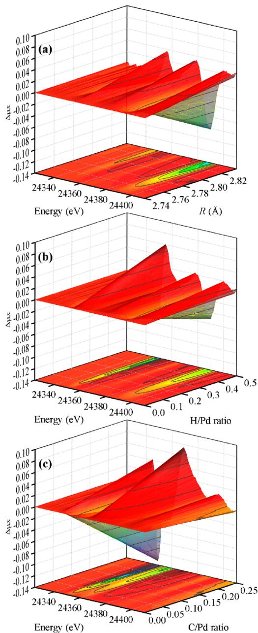
**Fig. 5.** Theoretical  $\Delta\text{XANES}$  spectra demonstrating the effect of the increase of interatomic distances (a), H/Pd (b) and C/Pd (c) ratios.
