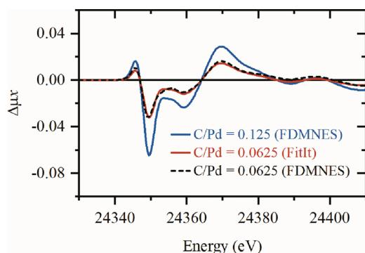
**Fig. 6.** Theoretical  $\Delta$ XANES spectrum for a C/Pd ratio of 0.0625, obtained by linear interpolation (red line) between FDMNES-calculated spectra for bare Pd (horizontal black line) and  $\text{PdC}_{0.125}$  (red line). The interpolated spectrum is compared with one directly calculated by FDMNES for the  $\text{PdC}_{0.0625}$  model (dashed black line) (For interpretation of the references to colour in this figure legend, the reader is referred to the web version of this article).
