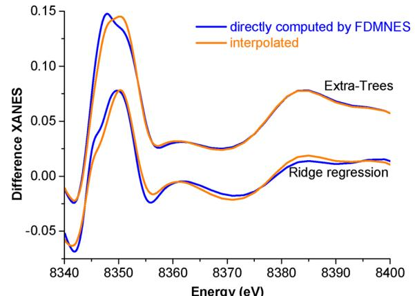
**Fig. 12.** Comparison between interpolated (orange) and exact (blue) difference XANES spectra for the CPO-27-Ni in interaction with CO, which differ from each other on the median error of interpolation. The difference spectra for Extra-Trees method were shifted vertically for clarity. (For interpretation of the references to colour in this figure legend, the reader is referred to the web version of this article).
